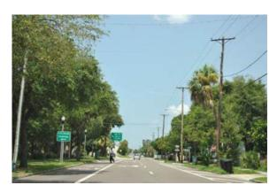
The operator of a vehicle traveling at 30 miles per hour along a residential street must observe the roadway beyond two (2) utility poles to see and safely stop for an impending danger.
